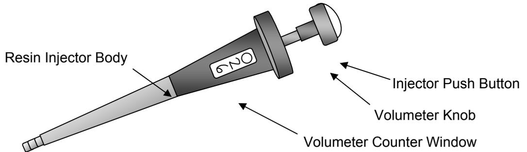
**Figure 7-26 – Resin Injector and Volumeter Counter Knob**
