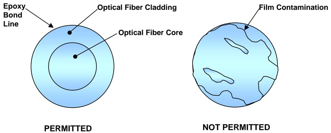
Figure 7-3 – Film Contamination of the End Face of an Optical Fiber
