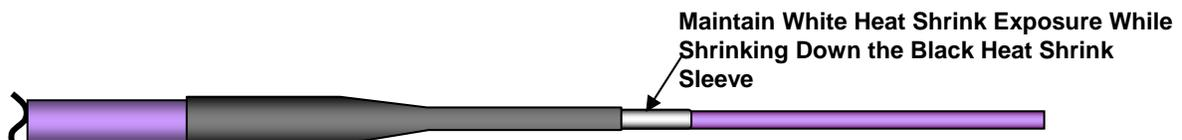
**Figure 7-20 – Installing White Heat Shrink Sleeve**
