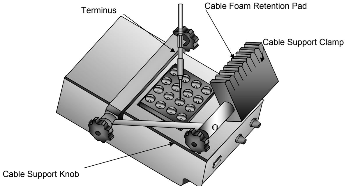
**Figure 7-39 – Curing Oven and Cable Support Clamp**
