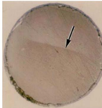
Figure 7-5 – Cracks on the End Face of an Optical Fiber
