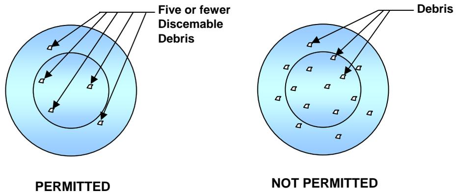
Figure 7-2 – Particle Contamination of the End Face of an Optical Fiber
