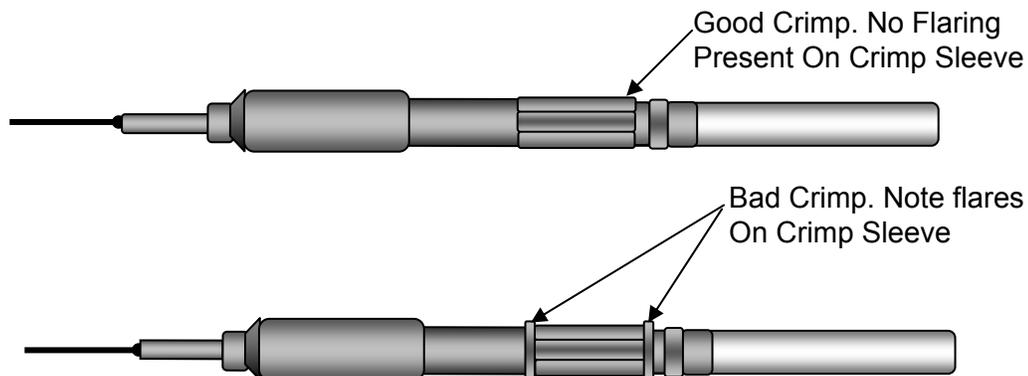
Figure 7-38 – Example of Good Crimp and Bad Crimp
