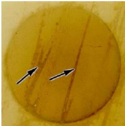
Figure 7-4 – Scratches on the End Face of an Optical Fiber
