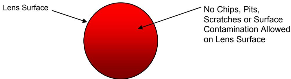
**Figure 7-7 – Visual Acceptance Criteria for Expanded Beam End Face at 10x Magnification**
