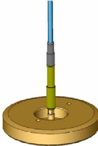
**Figure 7-41 – Inserting the Terminus into the Polishing Tool**
