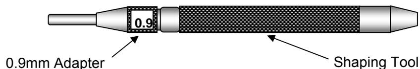
**Figure 7-31 – Installing the 0.9 mm Adapter onto the Shaping Tool**
