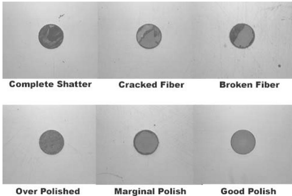
**Figure 7-6 – Visual Acceptance Criteria for Connectors at 200x Magnification**
